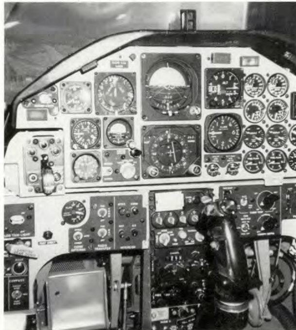
Modern simulators are fully instrumented. This T-38 simulator is almost an exact replica of the aircraft instrument panel.
