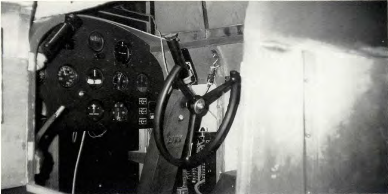
Early Link® trainers enabled students to practice only the fundamentals of instrument flight in a cramped cockpit.
